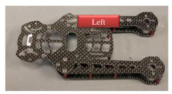
Figure 6 Attach each arm to the bottom plate
