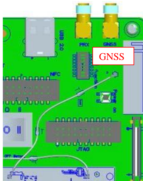
Figure 19 GNSS On Board PCB GNSS Antennas
